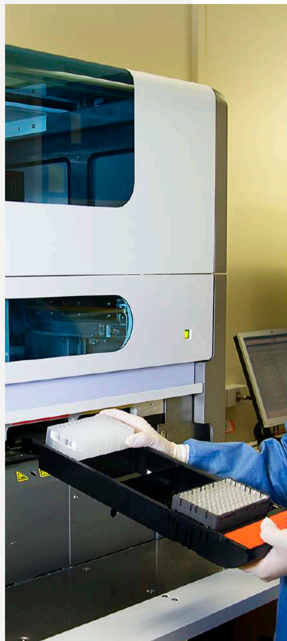
Nam Phan loading samples for nucleic acid extraction on Roche MagNA Pure 96
